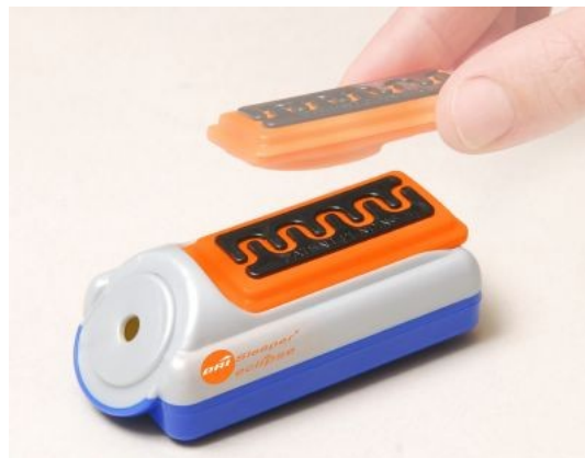
Figure 23. Dri-Sleeper wireless enuresis sensor.
